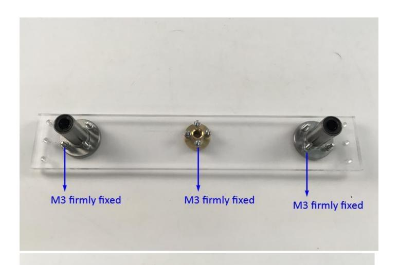
the yellow round center to the adge, one is long, another is short. when the rod go through the bearing, the long must be put inside and the short must be put outside.
