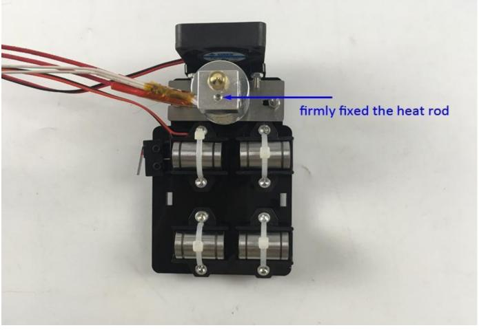
The temperature sensor is inserted into the specified hole, the screw is pressed against one of the threads, then firmly fix the screw, taking care not to damage the temperature sensor
