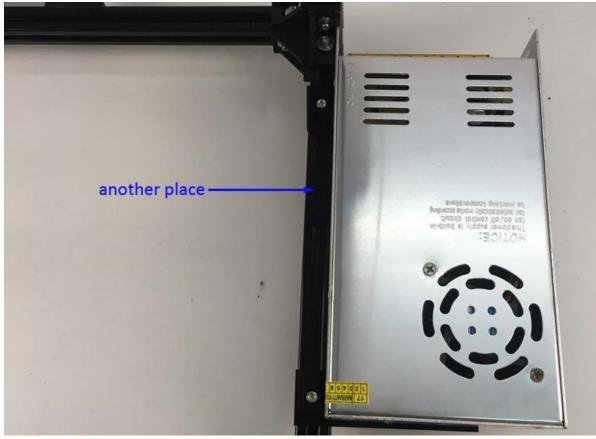
when use power, the safe is the most important!!! dont connect AC(110V or 220 V) to board directly. it's right connect the board to power, connect the board must be 12V.
