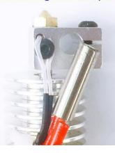
Insert the heating bar into the specified hole
