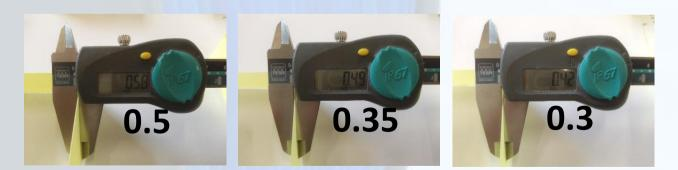
With an extrusion multiplier of 0.3, we achieve a layer width of 0.42mm. So we print the parts with a reduced flow of 70%.
