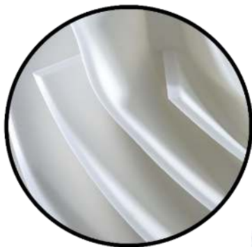
Close up a printed object with PLA-X³ (Printed on an Ultimaker 2+, 0.19 layer height, 242c)
