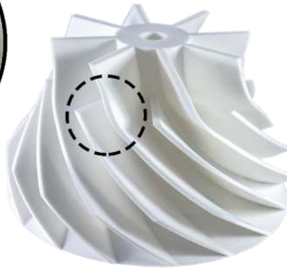
Close up a printed object with PLA-X³ (Printed on an Ultimaker 2+, 0.19 layer height, 242c)
