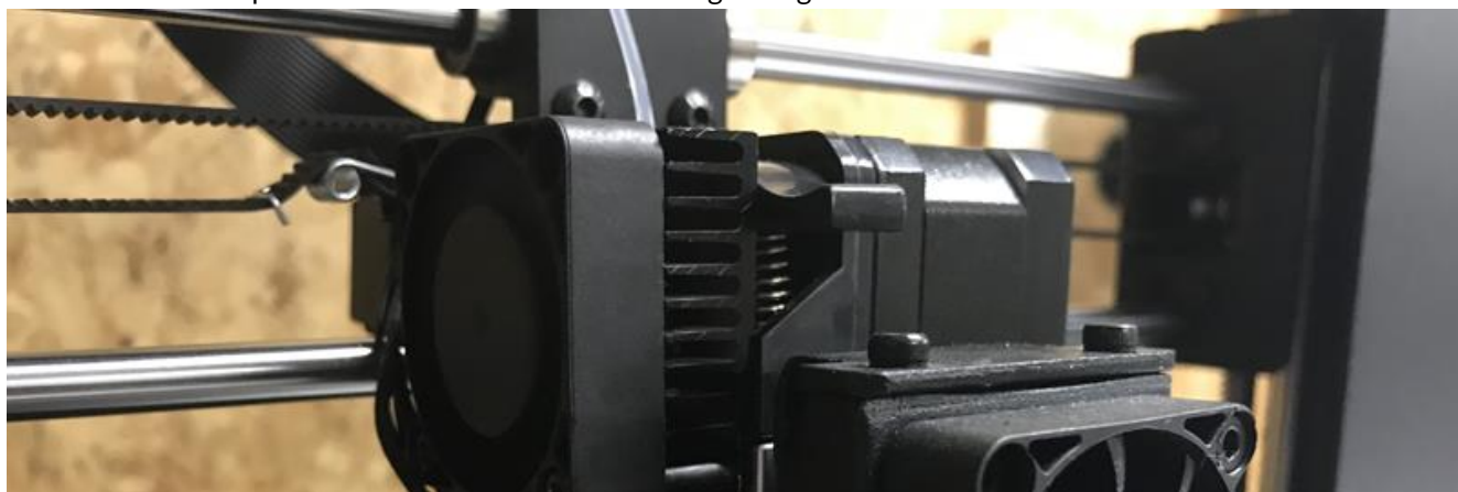
Example of a spring-loaded direct drive
